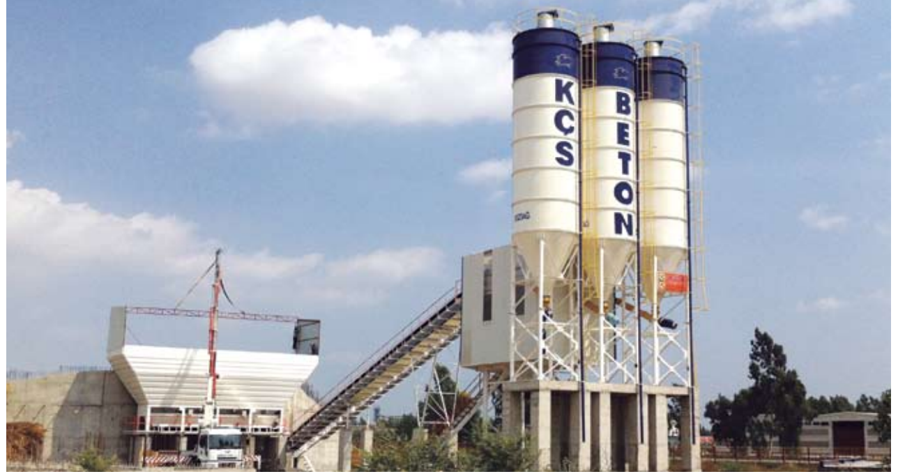
BS 240 240 m 3 /s Sabit Beton Santrali 240 m 3 /h Stationary Concrete Batching Plant
